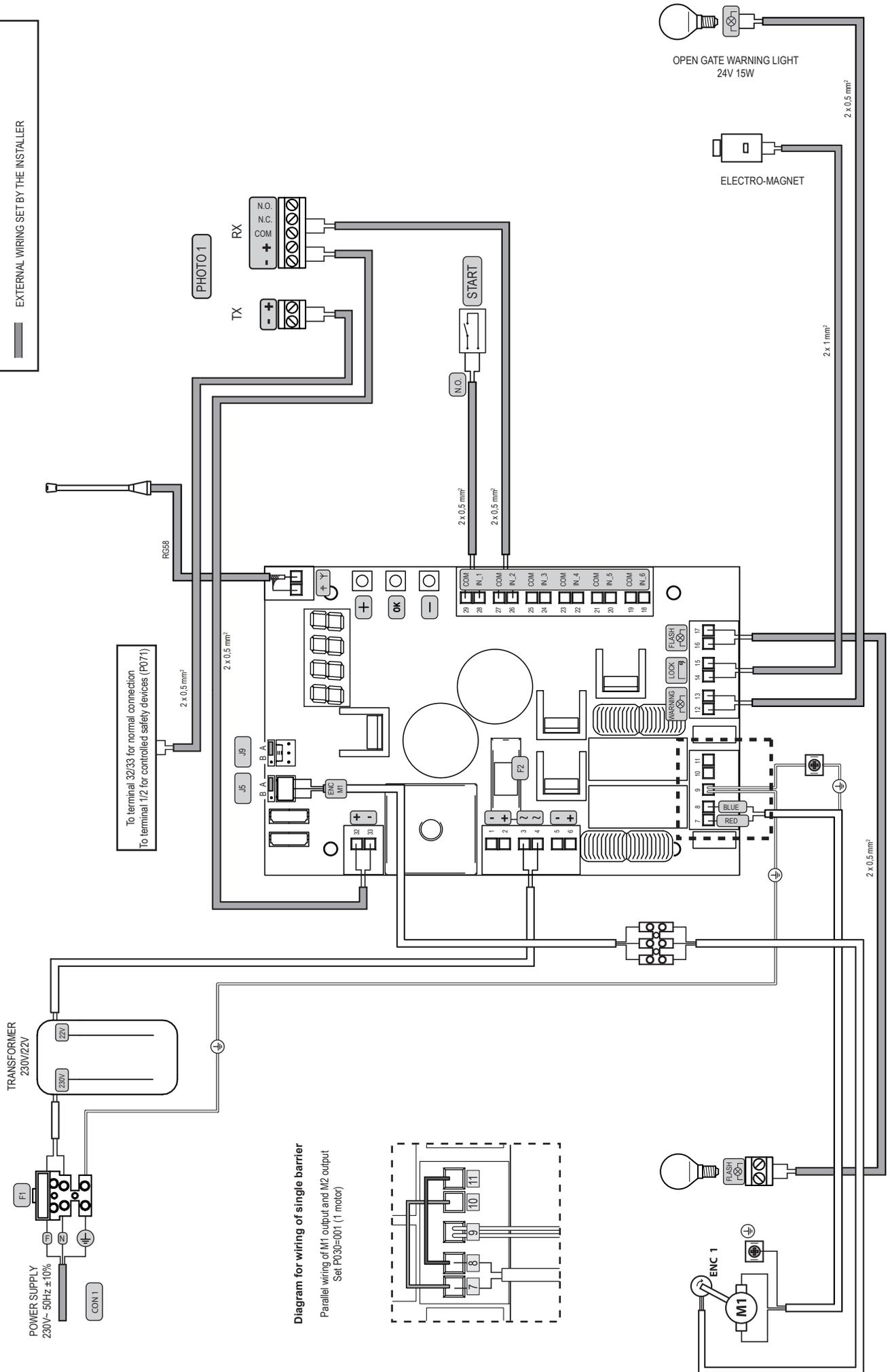
Diagram for wiring of single barrier
