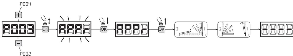
**WARNING (only Type 01 and Type 03)** Once you have executed the learning stroke, operate a complete cycle (opening/closing) and then check the manual release to make sure it is working properly. If it's to "hard" increase the value of P057 of 1 or more.
