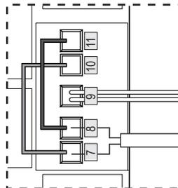
Wiring diagram for TYPE 01 (swing gate)
